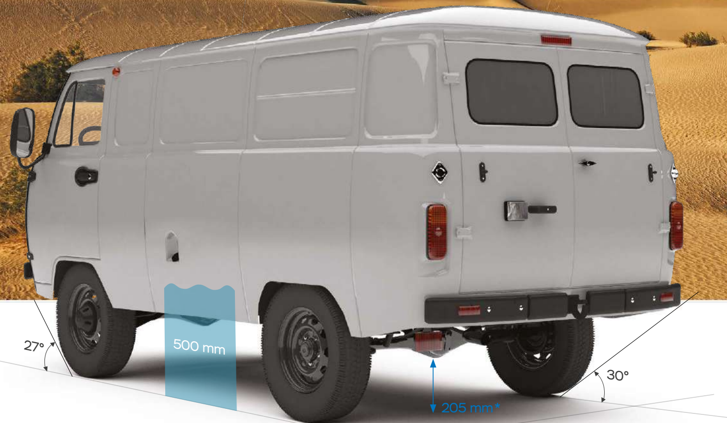
Minimum height of the chassis – distance from the ground to the axle housing.
