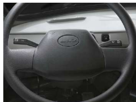
"Soft" steering wheel. Multifunctional Under-steering Switches
